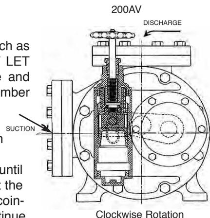
**STEP 3 -** For greater pressure, turn wrench to higher hole position. Each hole represents 20 PSI. **DO NOT EXCEED 6 holes.**
