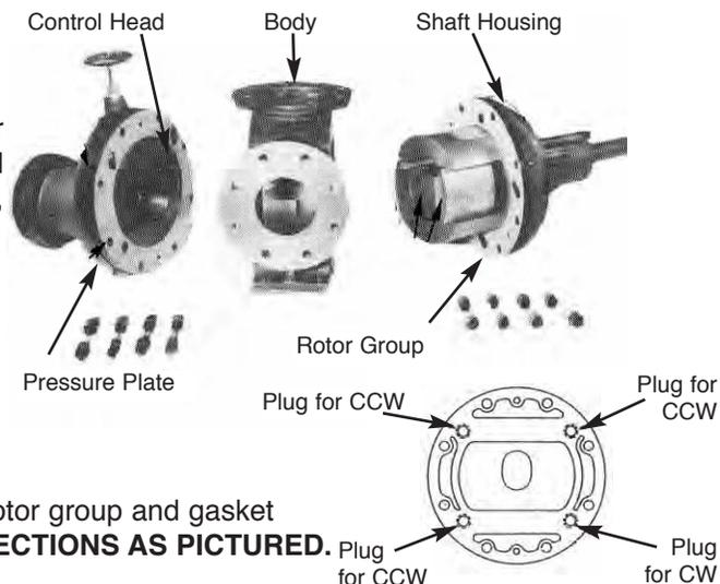
**STEP 4 -** Turn body “about face” and switch dowel pins.
