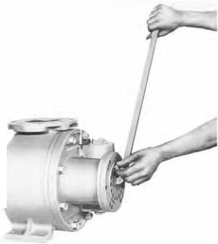
**STEP 2 -** To reset, pull wrench in direction of
