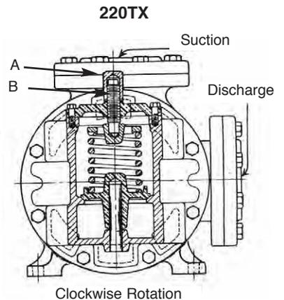
**STEP 1** - Unbolt bypass head and remove with bypass head gasket as one unit, making sure gasket is not damaged.
