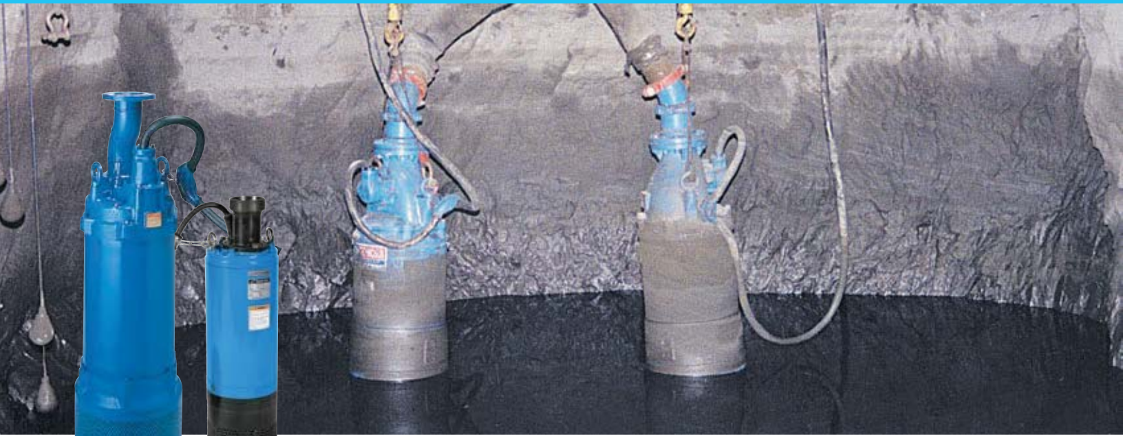
Slimline: LH33.0 - fits into 8" diameter pipes
